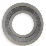
SERIES 9000 SOLID GASKETS - METAL GASKETS WITH INSERTS These gaskets are used, above all, on equipment with critical operating temperatures and pressures. The special shape of the solid metal gaskets with inserts combines the lasting stability of the solid part with the compensation, conformability and elastic recovery properties of graphite, even on existing system flanges.
